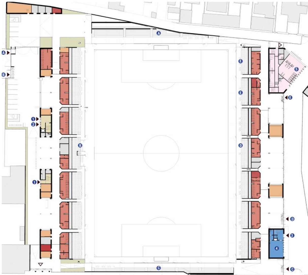
General Ground floor plan, showing concourses, and spectator facilities under stands, Community centre building located in top right corner.
